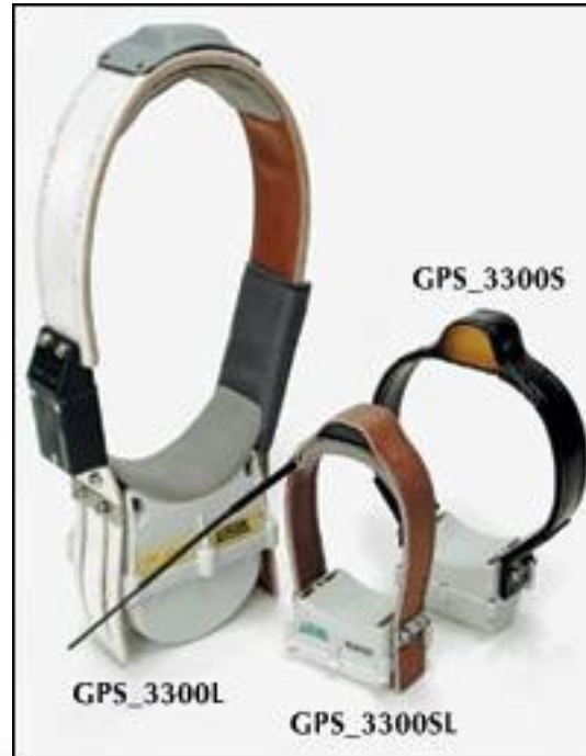
GPS collars with Store-on-board datalogging and a compact, light-weight design (190 gr) that's ideal for use on smaller animals.
